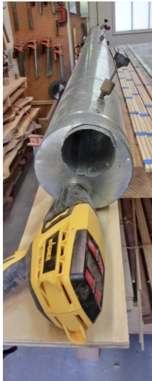
Figure 8: The oven for heat treating laminations
