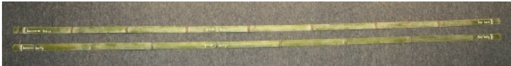
Figure 5: Bamboo laminations after preliminary shaping while still green. We see the positions of nodes relative to each other. The labeling with white out pen may seem excessive, as if you were elaborating instructions for an idiot. Exactly.
