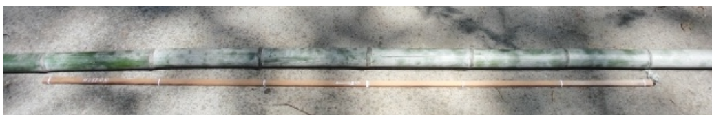
Figure 4: The nodes of this culm line up closely with the white marks of the "Nissun stick." This culm is a better than average find.
