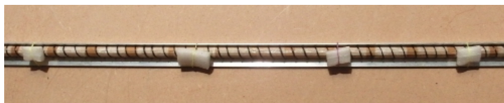
Figure 9: Layup "clamped" to straight L-bracket
