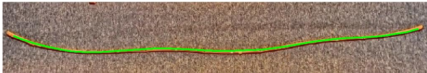
Figure 11: The design calculation of the unbraced shape (green curve) closely matches the actual unbraced shape. Some details: The braced tsuru tension that goes into this calculation is the measured value, 32.05\text{ kg} . The 1.5\text{ cm} elevation of the braced yumi centerline above the tsuru at the tips is important. If we neglect it, the computed Urazori shape is shallower by roughly 2\text{ cm} over much of the yumi’s length.
